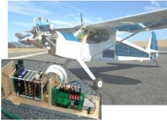
Fig. 8. UC Berkeley Sig Racal and PC-104 Payload
